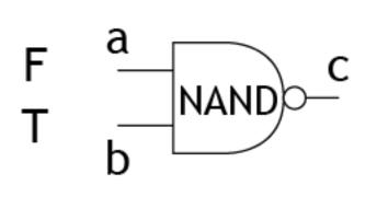
([a<sub>F</sub>,b<sub>F</sub>].c<sub>T</sub>)\* | ([a<sub>F</sub>,b<sub>T</sub>].c<sub>T</sub>)\* | ([a<sub>T</sub>,b<sub>F</sub>].c<sub>T</sub>)\* | ([a<sub>T</sub>,b<sub>T</sub>].c<sub>F</sub>)\* | a<sub>F</sub> | b<sub>T</sub>
