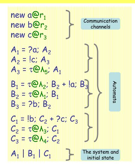
"Finite state" means: no composition or restriction inside recursion. Analyzable by standard Markovian techniques, by first computing the "product automaton" to obtain the underlying finite Markov transition system. [Buchholz]
