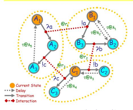
Communicating automata: a graphical FSA-like notation for "finite state restriction-free  $\pi$ -calculus processes". Interacting automata do not even exchange values on communication.
