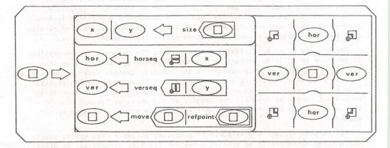
The little basic boxes composing the frame in the figure above have unitary size. Note that the reference point of the argument box has to be renormalized to the lower left corner (to place the frame in the correct position): the result of the refpoint operation is used to move the box.
