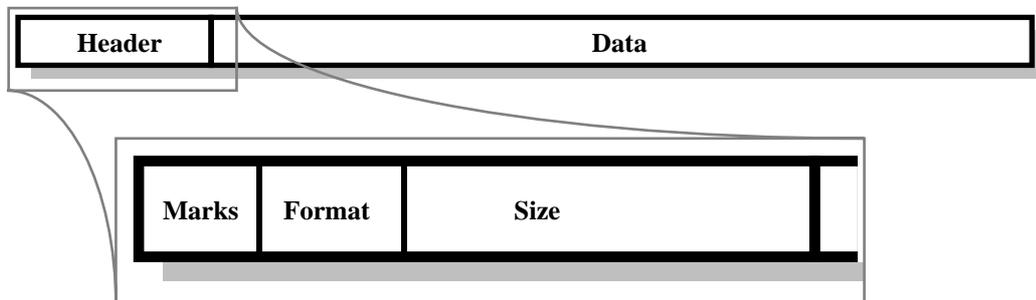
The header contains mark bits (the same as in unboxed words), a code indicating the format of the data section, and a size (number of items in the data section).
