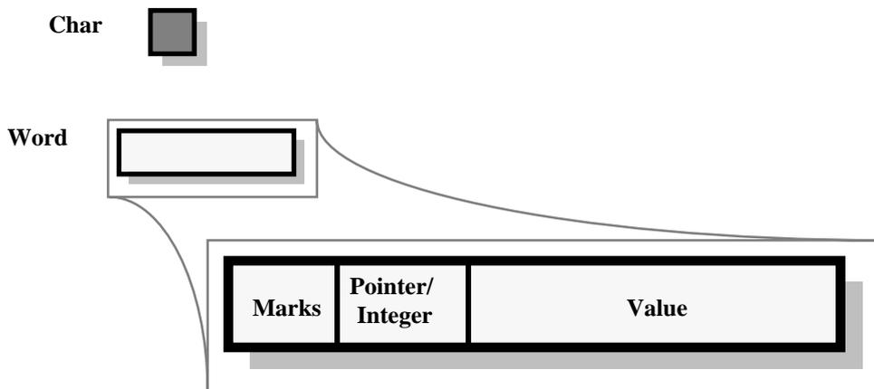
Unboxed words are further structured. They contain mark bits (used by the garbage collector and the persistence mechanism), a flag indicating whether this is an integer or a pointer (again, needed by the garbage collector), and an integer or pointer value.
