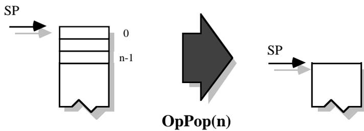
**OpSqueeze(n,m)** removes from the stack n elements, starting at depth m. **OpSqueeze(n,0)** is equivalent to **OpPop(n)**
