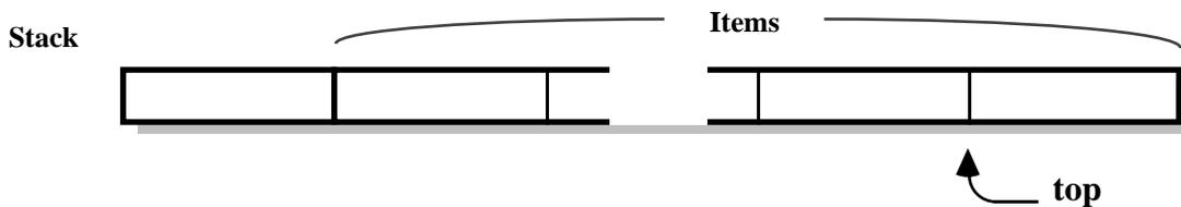
As stacks are used frequently in pictures, they are shown in the following space-efficient way:
