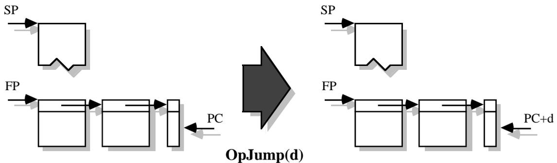
Conditional jumps are obtained by the **OpTrueJump(d)** and **OpFalseJump(d)** instruction, where  $d$  is a relative displacement from the current PC. Again, the exact meaning of  $d$  depends on implementations. **OpTrueJump** jumps if the top of the stack has the value true in it, otherwise proceeds to the next instruction. In both cases the top value is popped away. The following picture shows the two transitions for **OpTrueJump**; **OpFalseJump** is symmetric.
